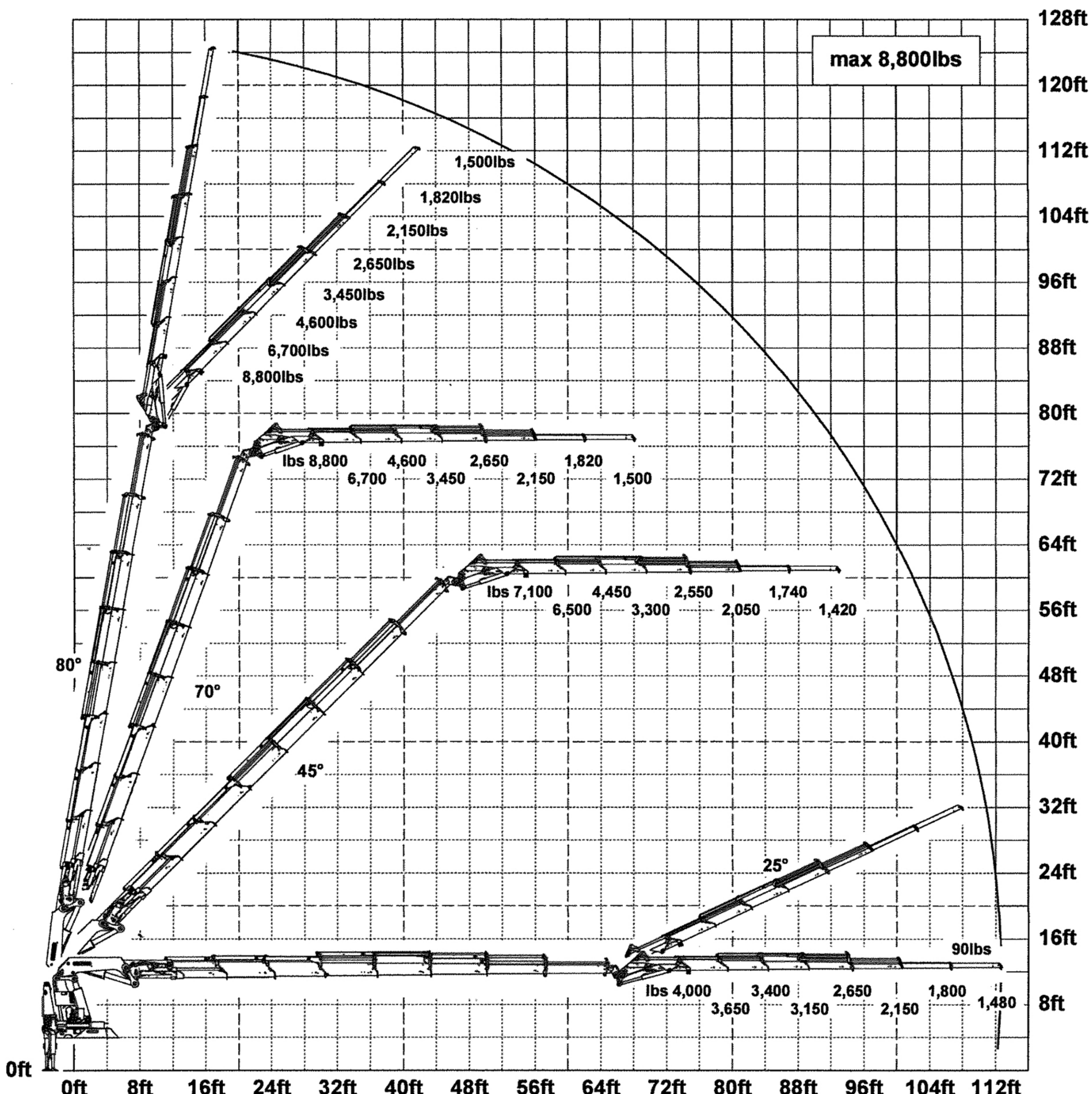
When using mechanical boom extensions, the loads shown on the charts need to be reduced by the weight of these extensions.
